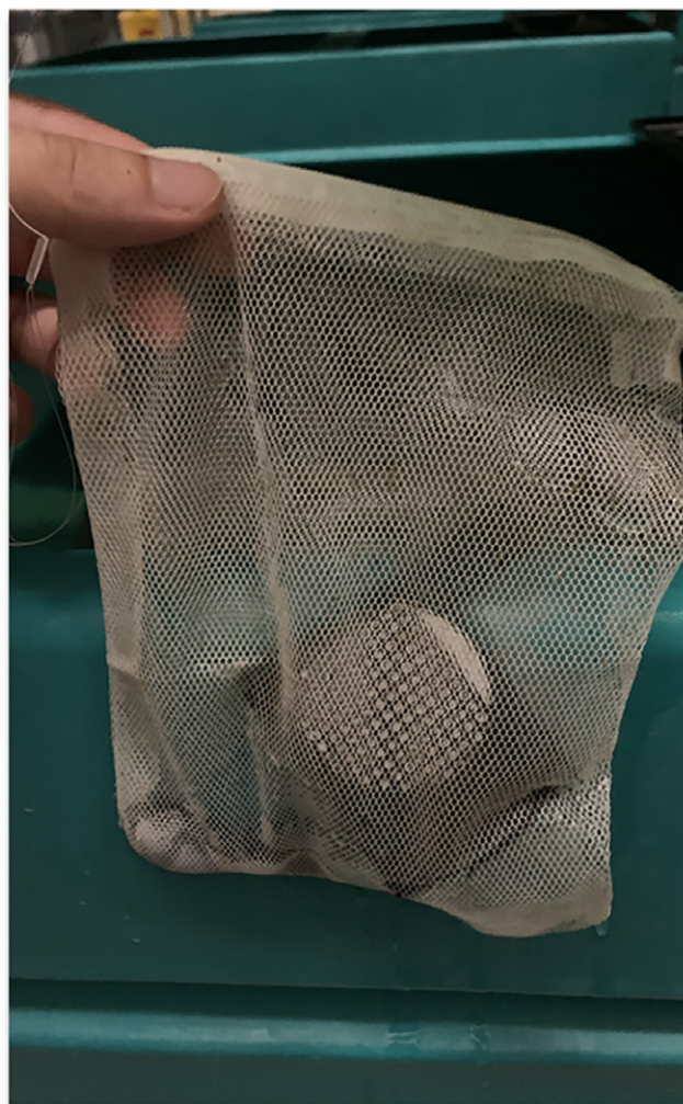
Figure 1. Example of filter assemblies placed in fish rack sumps. Depicted is a nitrocellulose (Nitro) filter, stabilized with a black, polyethylene plastic holder apparatus contained within a mesh polyethylene biofilter bag retrieved from a sump after its submersion period.
